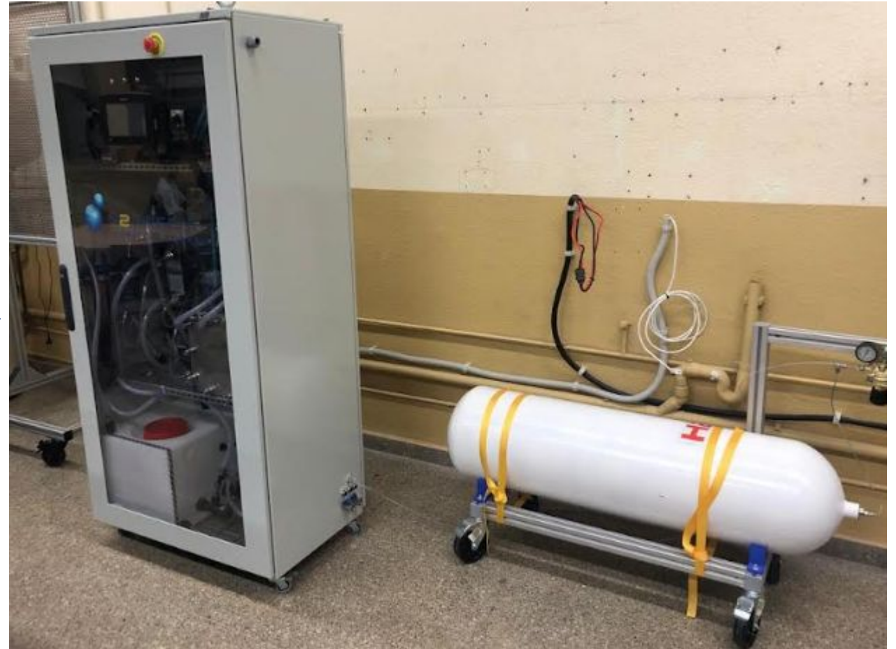
Electrolyzed 1KW, H 2 Green
